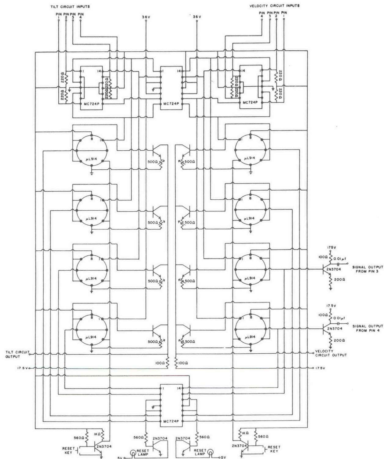
Fig. 19. Circuit diagram for velocity and tilt circuit.
